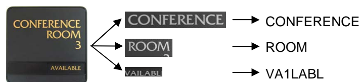
Figure 2: Steps of the optical character recognition: Color reduction, segmentation (left, middle), and optical character recognition (right)
