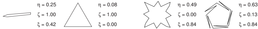
Fig. 8. Left: Two convex shapes with same extremum \zeta that can nevertheless be distinguished by their extent \eta and curvature \xi . Right: Two shapes with same curvature values \xi , but different extent \eta and extremum \zeta
