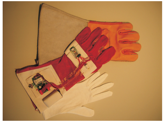
Figure 1: Layer-based wearing concept of the used data glove
